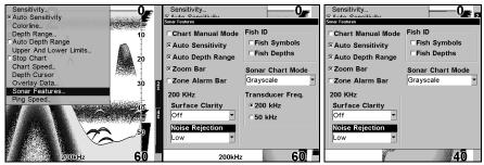
At left, Sonar Menu with Sonar Features selected. In the Sonar Features menu, Noise Rejection is selected with ASP in the default low setting (center, dual-frequency menu; at right, single-frequency menu).
